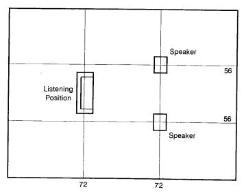
In our 14 by 18 foot example room, the thirds are 72 inches in the long dimension and 56 inches in the short dimension. The intersections of these measurements are used for third dimensions placement. In addition, the listening position is placed 72 inches from the rear wall of the room.
