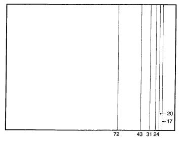
We use the same method to figure how far the centers of the speakers should be from the side walls. We take the width of the room, (14 feet) convert it from feet to inches,  $(14 \times 12 = 168)$  and divide the result by odd numbers.
