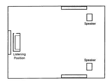
Bass problems that cannot be corrected with placement adjustments may be helped by the addition of bass traps or other bass control devices. Follow the instructions of the bass control devices as to their proper set-up and placement to correct the problems you are experiencing.
