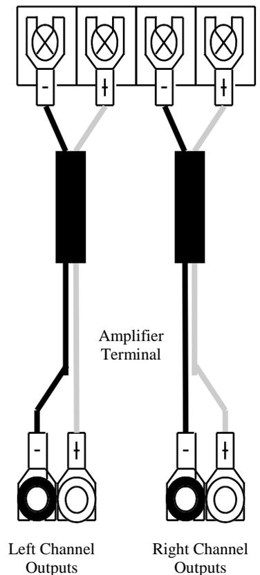
**Bare wires should never come into contact with the aluminum dress plate while the amplifier is on. Amplifier damage could result.**
